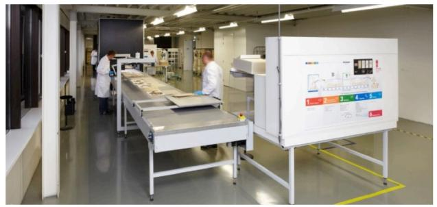
Figure 5. A "rapid scanning street" at the Naturalis Biodiversity Centre in The Netherlands is designed to digitize large collection at high quality and with low cost.
