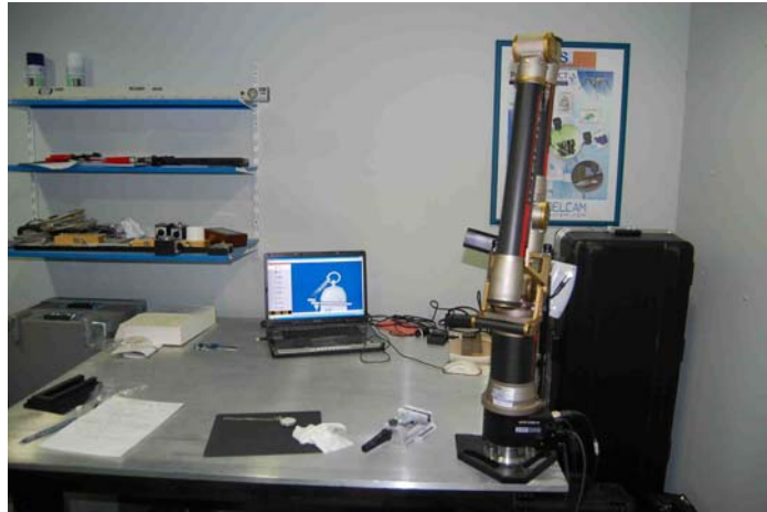
Image 8: Jointed arm (cimcore) and Laser head (METRIS)
